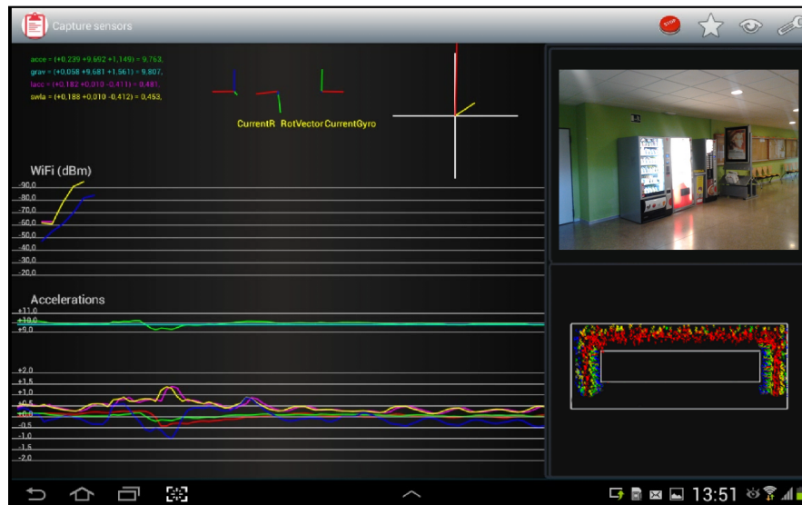
FIGURE 5.3: Main screen of our training application. The left side of the screen shows information from sensors measurements in real time as the operator moves throughout the scenario. On the right side it is shown the image visualized by the camera as well as an updated evolution of the particle filtering within the map.
